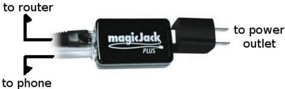
As you can see, it's very compact: less than 3" long, 2" wide, and weighs less than 2 ounces (very nice when you travel). There's a USB port with a plug at one end and an Ethernet jack and regular phone jack at the other end.
